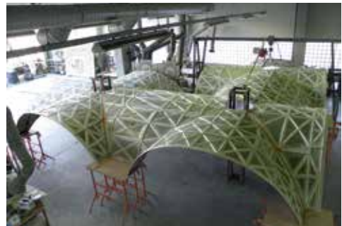
Fig. 8. New mosaic support of the vaults seen from above, subsequent to re-backing (photo ARM)
