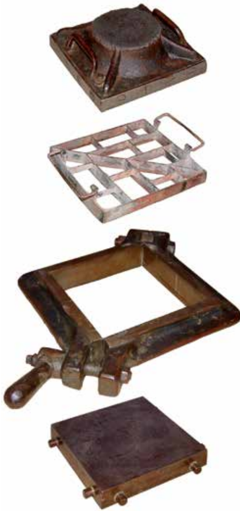
Fig. 3. Iron mold and metal alloy stencil for the manufacture of a hydraulic tile (Escofet 1886 S.A)
