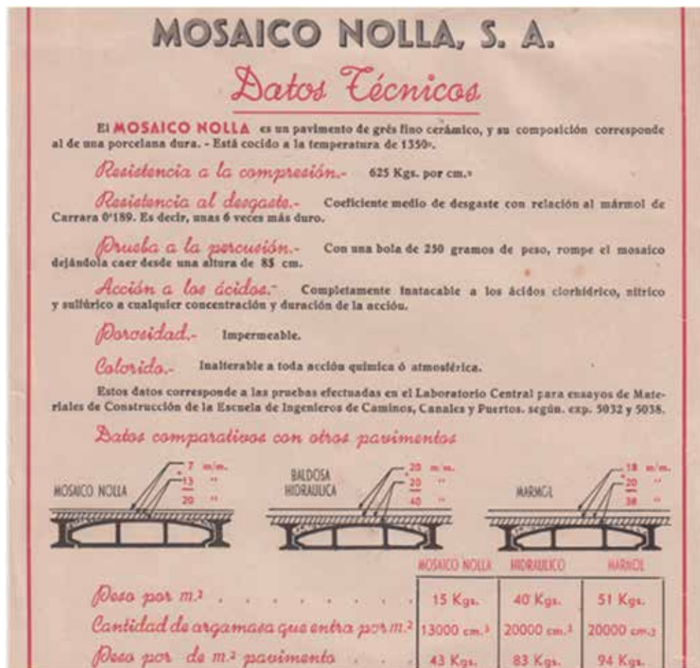
Fig. 6. Physical characteristics of Nolla tile, described in a factory catalogue (CIDCeN)
