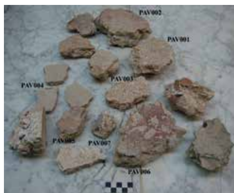
Fig. 2. Mortars recovered at Costa de la Serra, with the indication of the number of samples selected for our study (Photo by A. Bertral)
