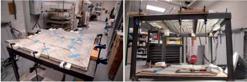
Fig. 4. Alignment of small corner sections on Plexiglas table top (photos C. Riccardelli, The Metropolitan Museum of Art)
