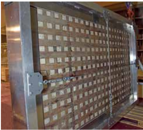
Fig. 5. Aluminium frame reinforcing the wooden cradle of the 19th-century restoration (photo Atelier de conservation-restauration, Musée départemental Arles antique)
