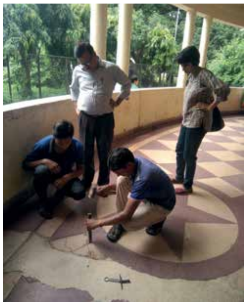
Fig. 3. Sampling an area of terrazzo flooring in a corridor, showing settlement, in All India Radio (Broadcasting House), Delhi (photo by Dandona and Shah)
