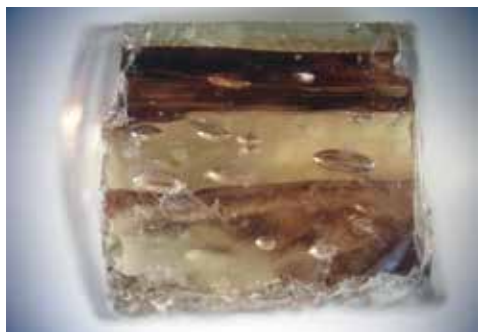
Fig. 4. Microscopic imaging of a detached gold-leaf tessera, side view (photo P. Loukopoulou, DCAMM, Hellenic Ministry of Culture and Sports)
