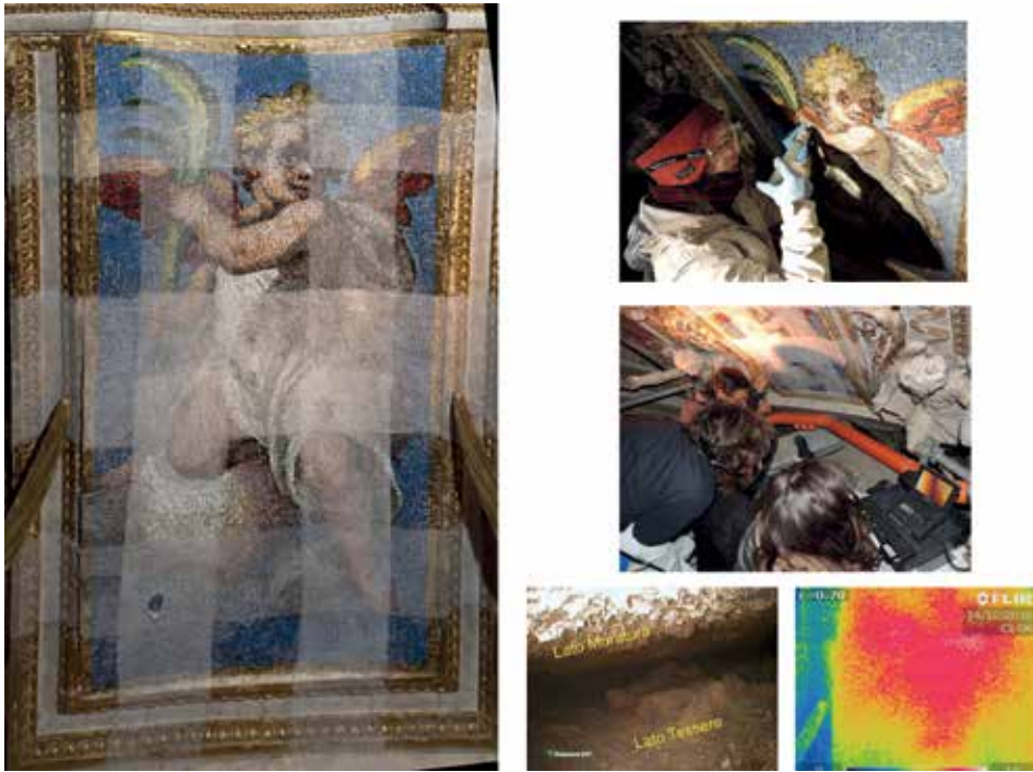
Fig. 10. Video-endoscopic investigation and consolidation during intervention on the left cherub (photo A. Rubino, R. Ciabattoni, © ISCR)
