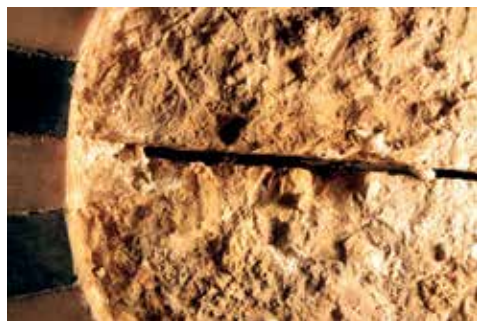
Fig. 4. Steleri of Istrian stone with marble tarsie laid over resin (photo E. Pannunzio).
