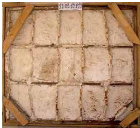
Fig. 2. Reverse side of a mosaic panel mounted on a plaster support (photo A. Ouslati)
