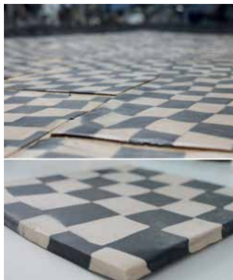
Fig. 7. Top - detail of the Temperance chapel ; Bottom - sample of unglazed semi-refractory ceramic (photo S. Vella)
