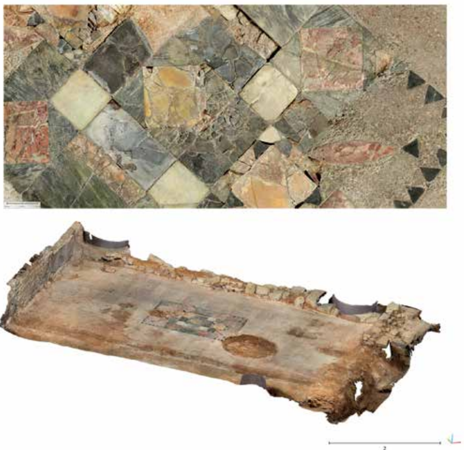
Fig. 3. Top: orthomosaic with 0.0003m GSD; Bottom: textured 3D model (photo by authors)
