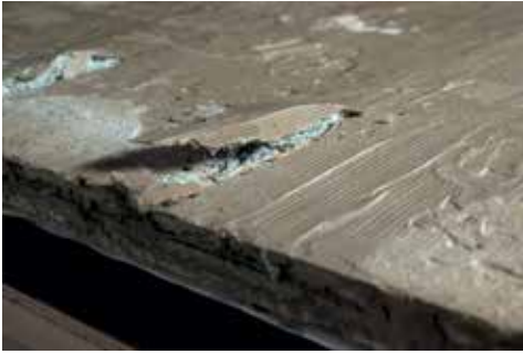
Fig. 9. Reverse side of the lower proper left corner mosaic panel, showing corroded aluminium bar and lifting section of epoxy, 2017 (photo J. Chloros)
