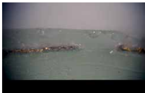
Fig. 3. Perfect bonding of the two glass layers due to the lack of gold
