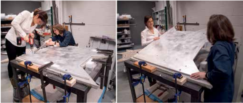
Fig. 5. Beth Edelstein and Rebecca Gridley drill holes using the composite panel as a drilling template (photos C. Riccardelli, The Metropolitan Museum of Art)
