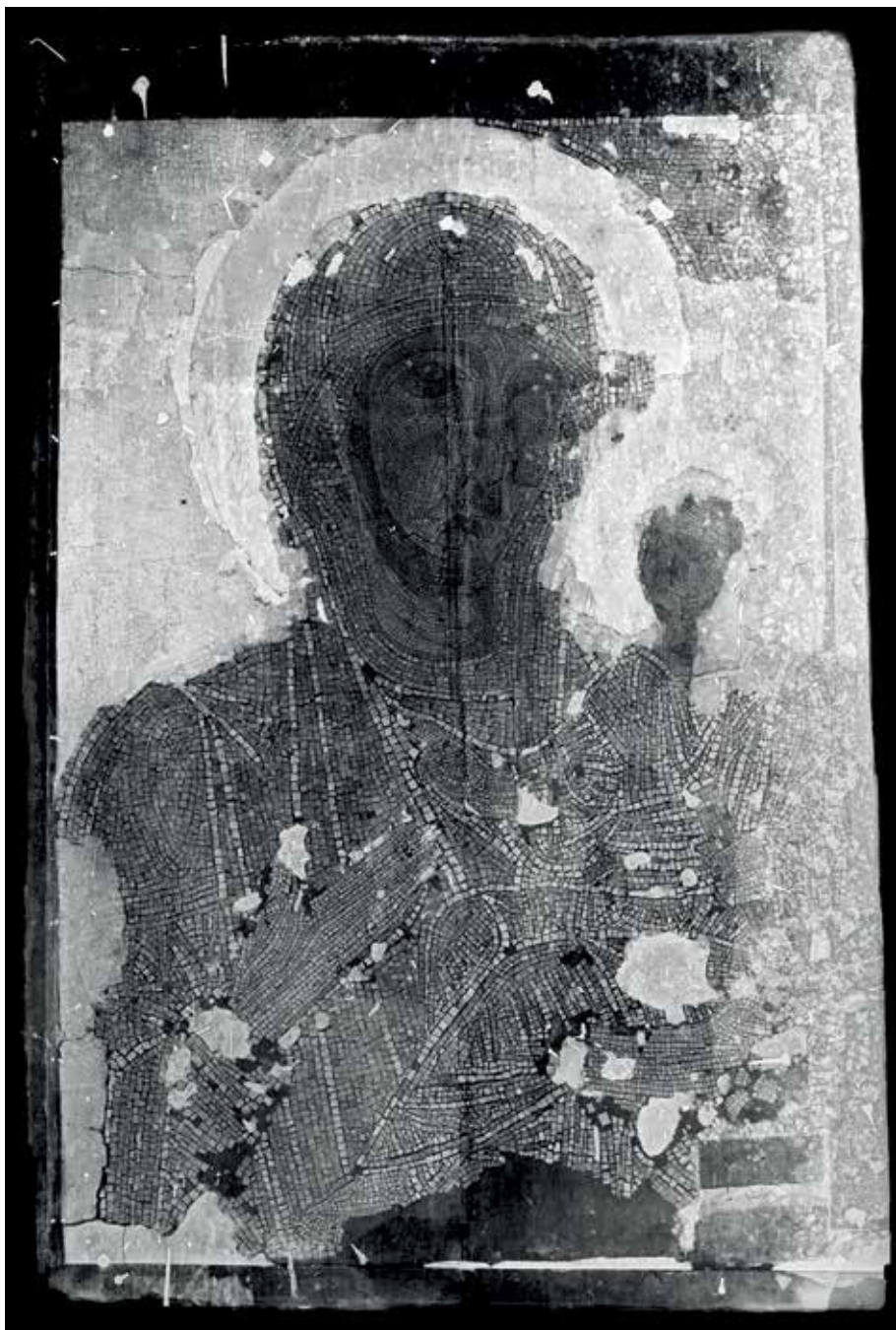
Fig. 6. X-Ray image of the icon, 15 sections merged and enhanced in Photoshop, Energy 55-60kV, Tube Current 0,2-0,63mA, Exposure Time: 20sec-3mins
