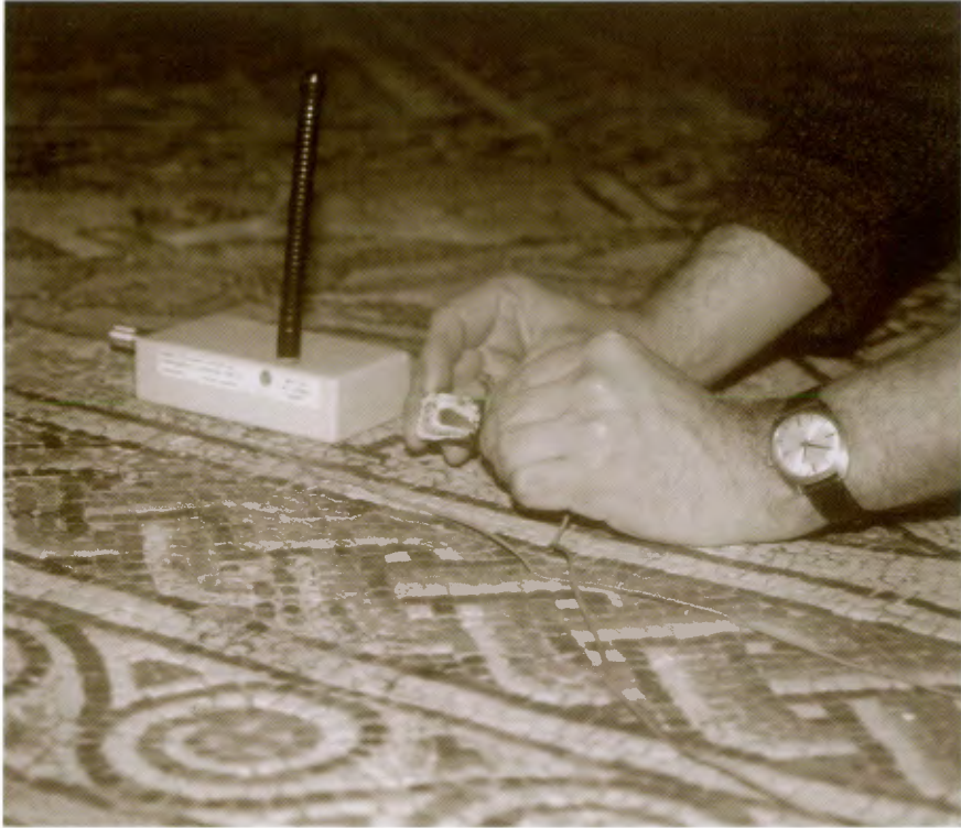
Fig. 4 : Application of a surface temperature sensor to the mosaic, attached to the radio transmitter by means of a cable.
