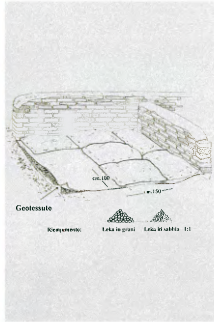
Fig. 4 : Seasonal protection for the winter period made of direct application of “cushions”. This system consents the easy removal for late spring and summer seasons.
