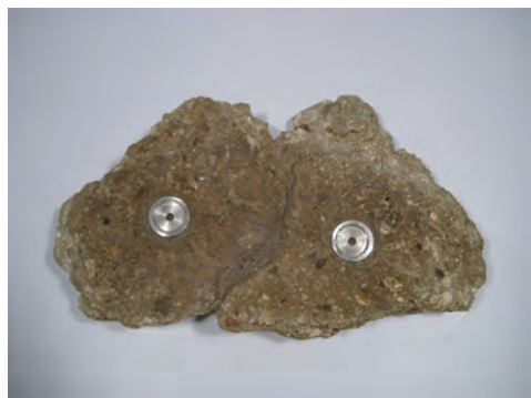
Fig. 8. Magnets implanted in the mosaic mortar (photo: Manlio Titomanlio)
