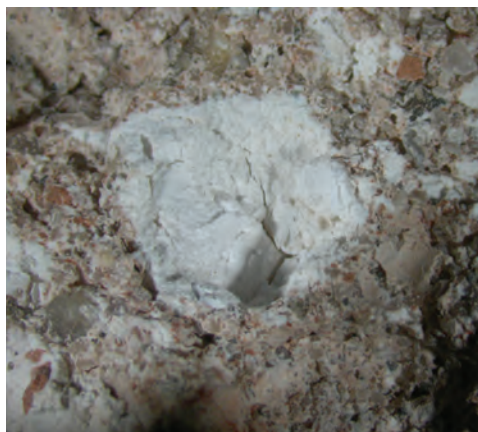
Fig. 7. 'Kalkspatzen' - detail of the first layer of nucleus (Photo: Brigitta Maria Kürtösi)
