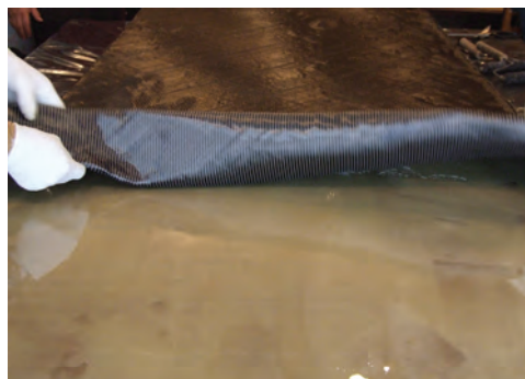
Fig. 9. The preparation of the new support with woven carbon fibre and 3PSP2 resin (Photo: Brigitta Maria Kürtösi)
