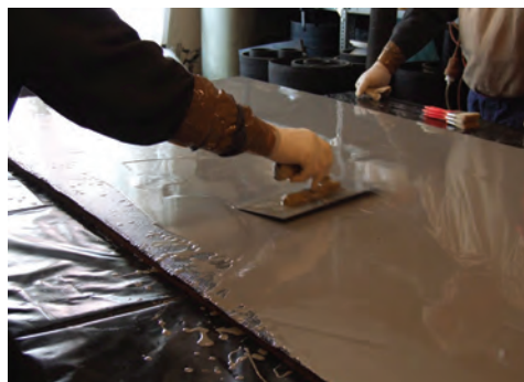
Fig. 10. The preparation of the new support with woven carbon fibre and 3PSP2 resin (Photo: Brigitta Maria Kürtösi)
