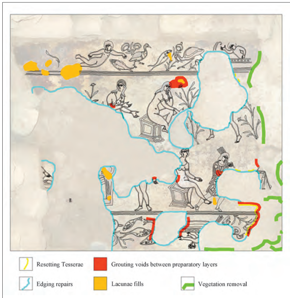
Fig. 13. Condition assessment-surface and biological deterioration (Drawing: the team)
