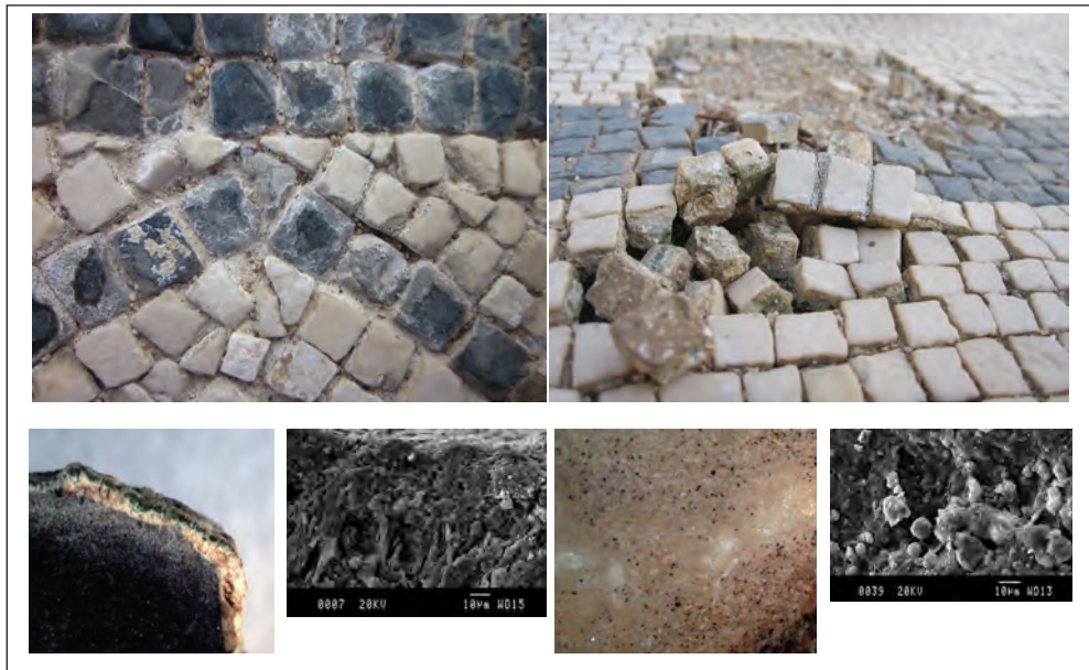
Fig. 8. Areas affected by microbiological growth and the resulting bulging issues; and close-ups of the microbiological growth and scanning-electron microscope photomicrographs of both a white and black affected tessera (photos: Sílvia Llobet, Patrimoni 2.0 Consultors SL)
