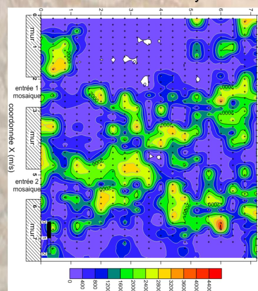
This Mosaic showed a substantial alteration especially near the surface. The small islands characterized by high velocity values match the highly compacted areas which represent lacunas repaired with cement based mortar
