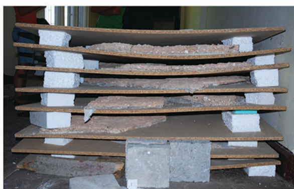
The considerable weight of the fragments had caused significant deformation of the working tables
