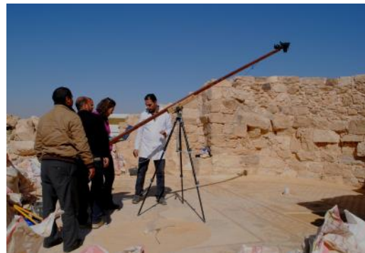
Fig. 4: A low-cost custom-made crane was installed on site for the photographic documentation of the mosaic floors.
