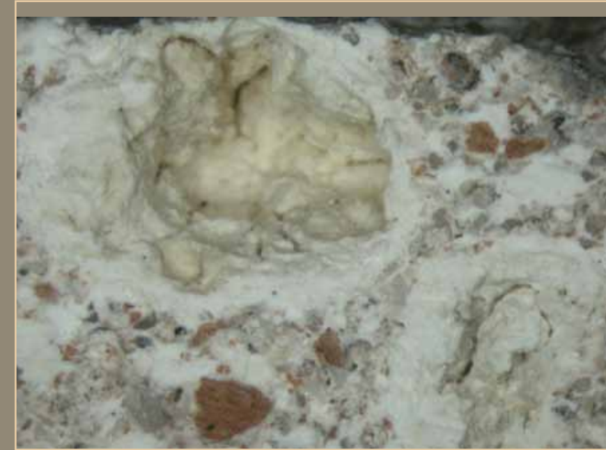
"Kalkspatzen" - detail of the second layer of the nucleus
