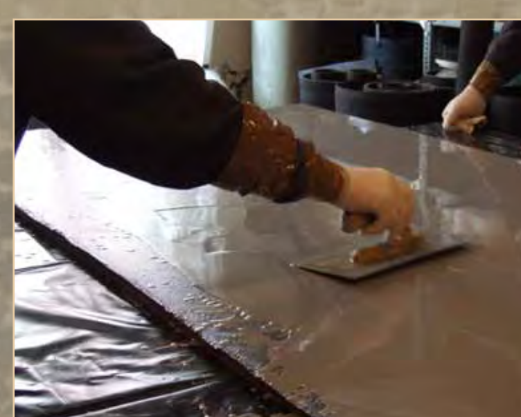
The preparation of the new support with woven carbon fibre and 3PSP2 resin
