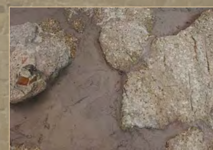
Levelling of the backside of the mosaic was made by the lightweight lime-based mortar ( above )
